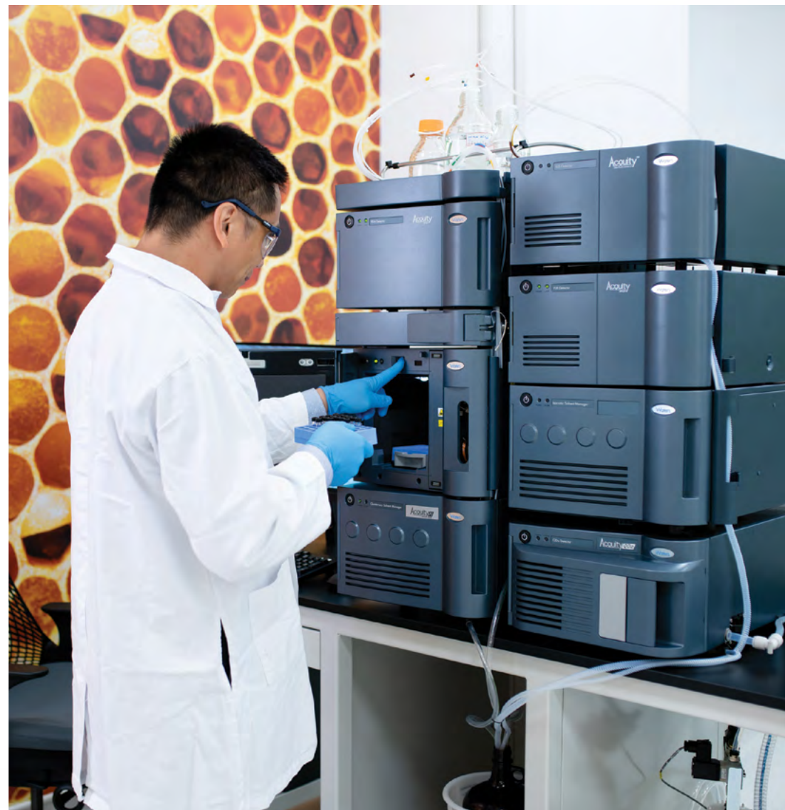
ACQUITY UPLC H-Class PLUS System with ACQUITY QDa Mass Detector and multiple optical detectors.
