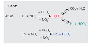
The eluent counter ions are also replaced with hydrogen carbonate. The carbonic acid that is produced in this way is unstable and only weakly dissociated, meaning that a lower background conductivity is measured than would be found with the non-suppressed eluent. Depending on the eluent composition, background conductivity values of approximately  $0.8-1.2 \ \mu$ S/cm are typical for chemical suppression.
