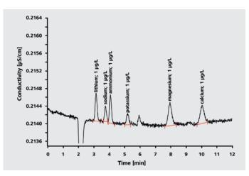
**Determination of 1 µg/L standard cations in ultrapure water** Column: Metrosep C Supp 1 - 150/4.0; eluent: 5 mmol/L HNO<sub>3</sub> + 50 µg/L Rb<sup>+</sup>; column temperature: 40 °C; sample volume: 20 µL; flow rate: 1.0 mL/min, conductivity detection with sequential suppression
