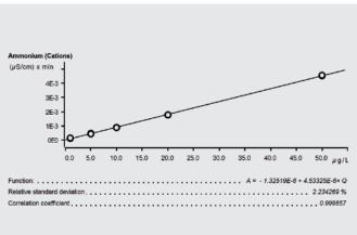
**Ammonium, linear calibration of 1–50 µg/L, 3 injections per level** Column: Metrosep C Supp 1 - 150/4.0; eluent: 5 mmol/L HNO<sub>3</sub> + 50 µg/L Rb<sup>+</sup>; column temperature: 40 °C; sample volume: 20 µL; flow rate: 1.0 mL/min, conductivity detection with sequential suppression
