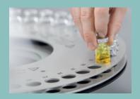
Heating vial by vial, the water contained in the samples is evaporated. A constant stream of an inert carrier gas is used to bring the water fraction into the titration cell, where it is determined. The sample matrix stays in the vials, which are simply disposed of
