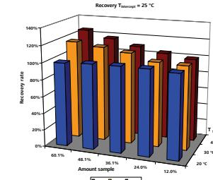
Increasing the temperature of the measuring solutions gives higher signals while the correlation coefficient decreases.
