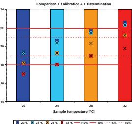
The resulting signal and curve shape of a dilution titration is influenced by the temperature of the measuring solution.
