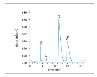
Sample: drinking water; column: Metrosep C 4 -100; eluent: 1.7 mmol/L HNO3, 0.7 mmol/L DPA; temperature: 25 °C, flow: 0.9 mL/min.
