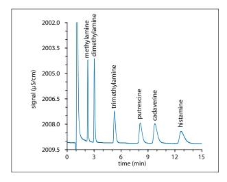
Sample: biogenic amines (5 mg/L methylamine, 10 mg/L of each dimethylamine, trimethylamine, putrescine, cadaverine and histamine); column: Metrosep C 4 - 100; eluent: 6 mmol/L HNO<sub>3</sub>; temperature: 25 °C, flow: 0.9 mL/min.
