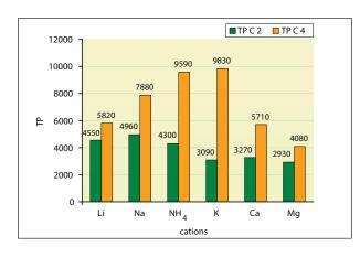
Separation of the standard cations with Metrosep C 4-150 and Metrosep C 2-150 – comparison of plate counts. The markedly improved peak shapes result in higher plate counts, which allows for lower detection limits for the Metrosep C 4.
