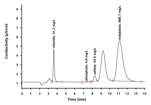
Molybdate protects the heating system and is added as a modifier. It can be quantified directly with the standard anions in a determination.
