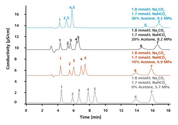
The backpressure increases gradually as acetone content increases. The pressure is 6.9 MPa at 10%. The retention time of phosphate and sulfate increases when adding acetone. The monovalent anions elute earlier. From 20% acetone content, chloride and nitrite as well as bromide and nitrate co-elute.
