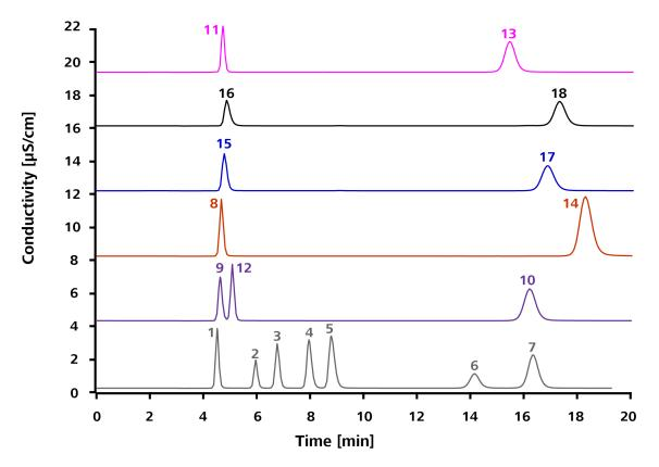
MSA and formate show a good separation with fluoride. Oxalate shows a good separation with sulfate. The separation of formate/acetate is not sufficient.
