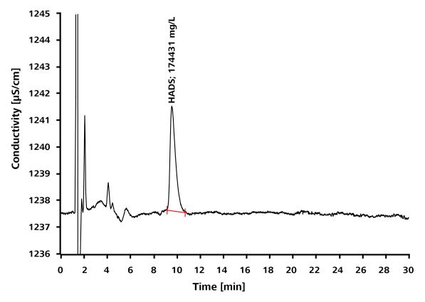
In these measuring conditions, all standard anions elute under 3 minutes and do not disrupt the determination.
