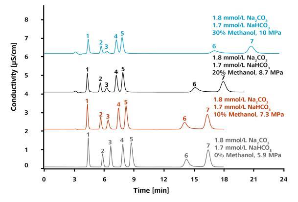
The backpressure increases gradually as methanol content increases. The pressure is 7.3 MPa at 10%. The retention time of phosphate and sulfate increases when adding methanol. The retention time of the monovalent anions decreases only slightly. Increasing the methanol content results in a weaker detection of nitrite. An interference peak forms at the injection peak with increasing solvent content.
