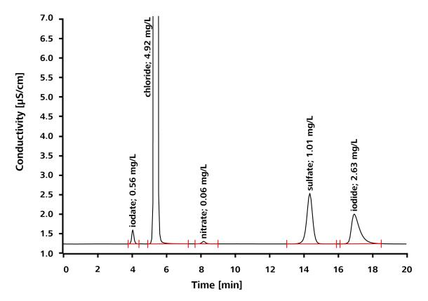
Fluoride elutes at the same retention time as iodate. If the sample contains fluoride, it is advisable to confirm the iodate with UV detection.
