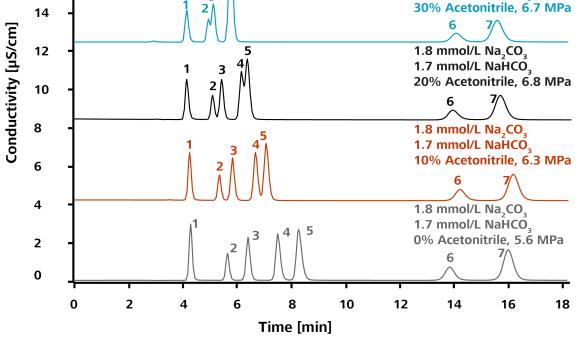
The pressure is 6.3 MPa at 10%. The monovalent anions elute earlier. At 20% acetonitrile content, chloride and nitrite as well as bromide and nitrate co-elute. Acetonitrile as organic modifier generates the smallest backpressure.
