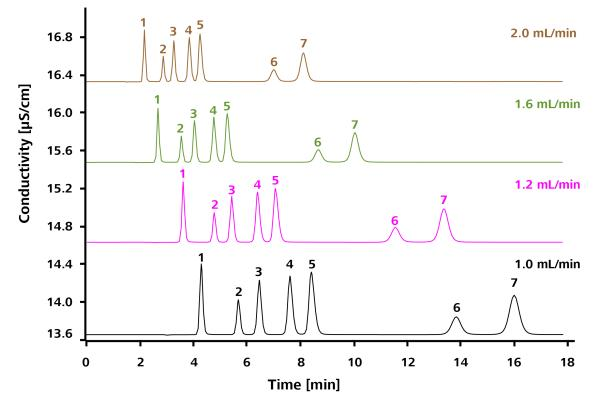
The retention times of all standard ions decrease with increasing flow rate. Fluoride approaches the injection peak.
