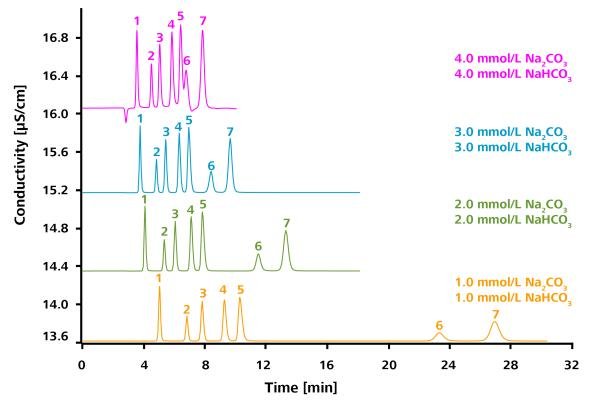
The retention times become shorter with increasing sodium carbonate / sodium hydrogen carbonate concentration. Those for the polyvalent anions phosphate and sulfate are strongly shortened in particular. With 4 mmol/L sodium carbonate, 4 mmol/L sodium hydrogen carbonate, phosphate co-elutes with nitrate.
