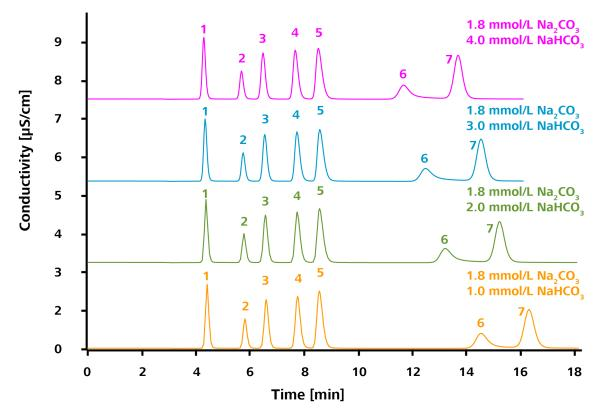
When the sodium hydrogen carbonate concentration is increased, the retention time of the monovalent anions decreases only slightly. For phosphate and sulfate, however, the retention time decreases evidently.
