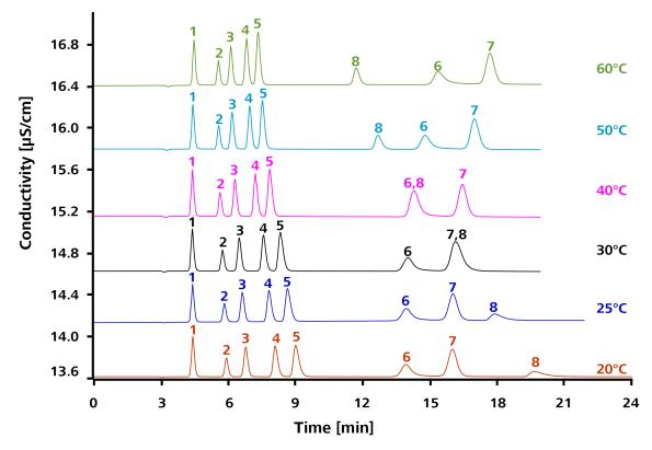
An increase in temperature results in slightly shorter retention times of the monovalent anions. The retention time of iodide, however, is drastically reduced when increasing the temperature. Iodide co-elutes with sulfate at 30 °C and with phosphate at 40 °C. At a higher temperature, phosphate and Sulfate elute later.
