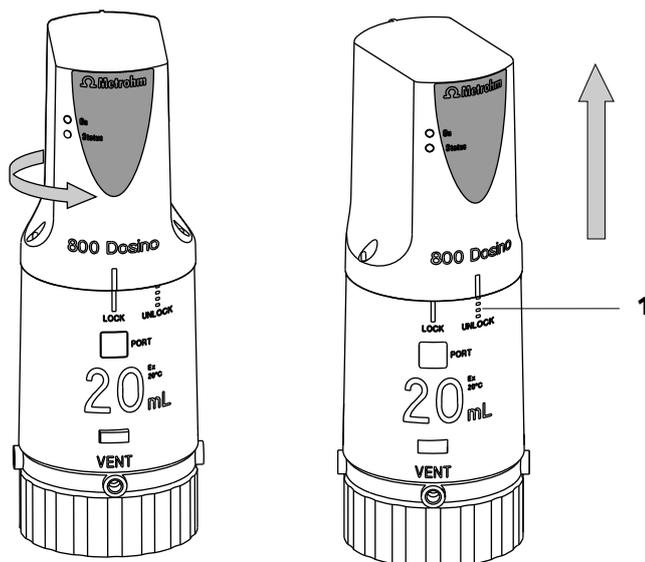
Figure 18 Removing the 800 Dosino from the 807 Dosing Unit
