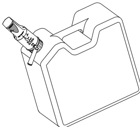
Figure 4 800 Dosino on the canister
