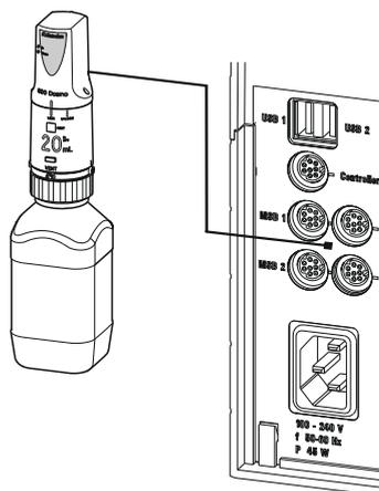
Figure 9 Connecting the 800 Dosino to the Titrando
