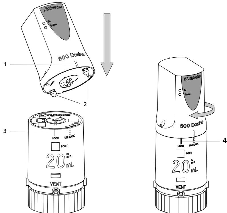
Figure 16 Mounting the 800 Dosino onto the 807 Dosing Unit
