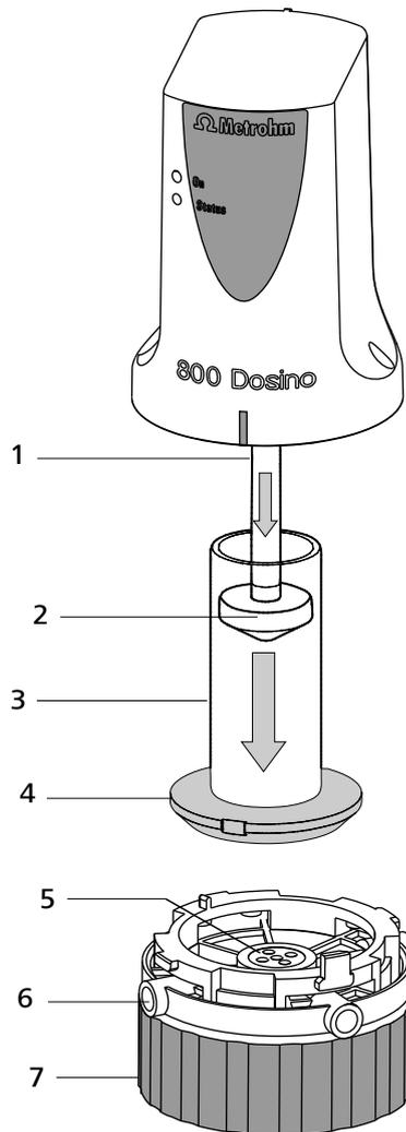
Figure 10 Dosing / Filling of the dosing cylinder
