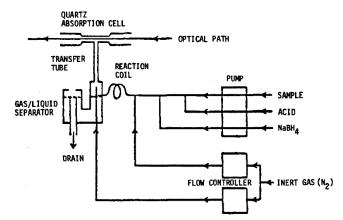
Figure 1. Schematic diagram of vapor generation accessory.
