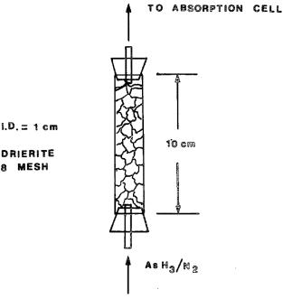
Figure 2. Glass trap with eight mesh drierite.
