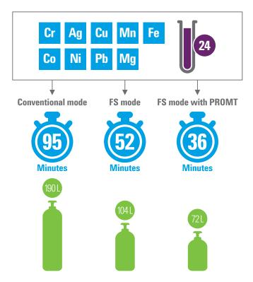
Nine elements in 24 samples were quantified in three different ways: Conventional FAAS mode (3 integrations of 3 seconds for each element), Fast Sequential mode, and Fast Sequential mode with PROMT acquisition. The analysis used an autosampler, included a Calibration Zero and three standards. A 5 s rinse was performed every 10 samples.
