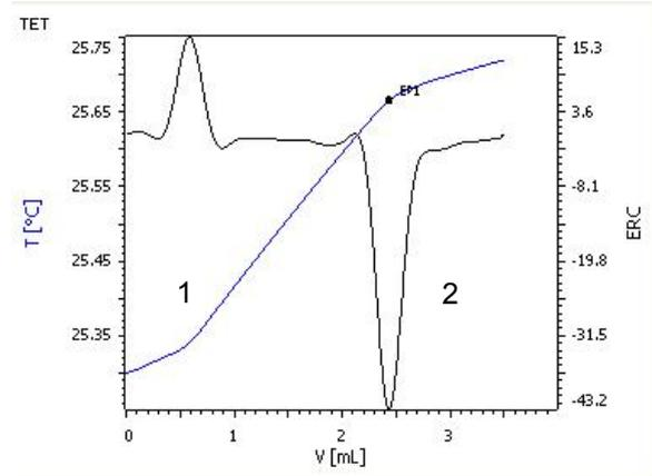
*Standardization of Al-K titrant with NaCl solution*
