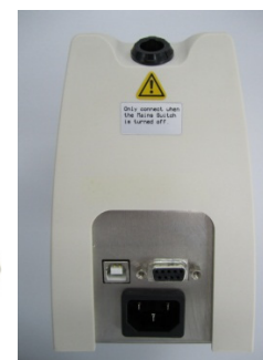
Figure 6: Polytron version 3 – rear view control unit.
