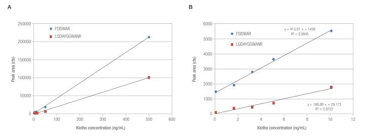
Figure 2. Calibration curves for the detection of Klotho from plasma using SMART Digest IA Streptavidin kit. Samples were run in triplicate. Figure 2A shows the full range of the calibration curve. Figure 2B shows the lower concentrations with linear fit.
