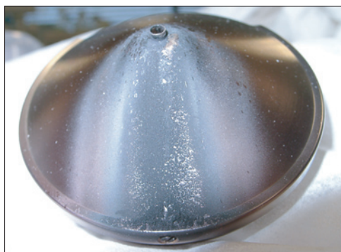
Figure 2: Ion sweep cap after several hundred injections, showing contamination from red wine
