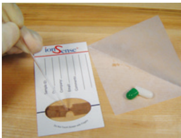
Figure 4. OpenSpot cards used for liquid and solid sample application
