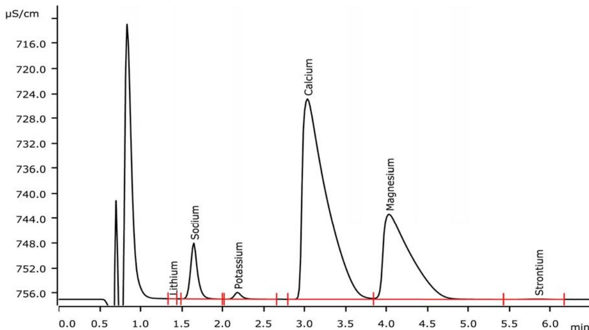
Reducing the analysis time is a demanding task because peak resolution is the limiting factor. With a microbore column of 100 mm length, standard cations in tap water can be analyzed within only 5 minutes. Strontium can also be determined by simply extending the run time to 6.5 min.
