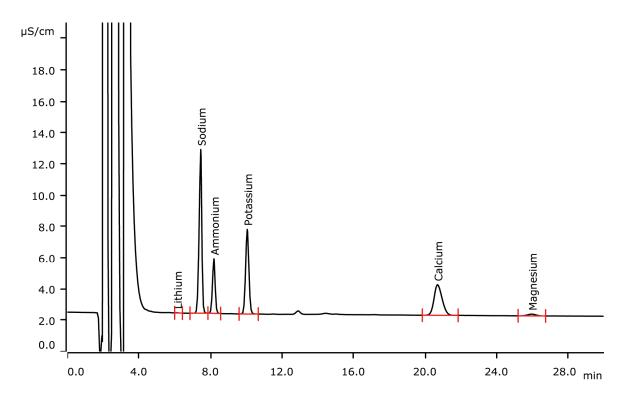
Cleanliness is an indispensable condition in production of electronics. Especially ionic contamination can reduce the quality of products. Here, the determination of cations on the surface of circuit board materials is shown. The method applies intelligent Partial Loop Technique (MiPT) from one sample to both anion and cation channel. See AN-S-317 for anion determination.
