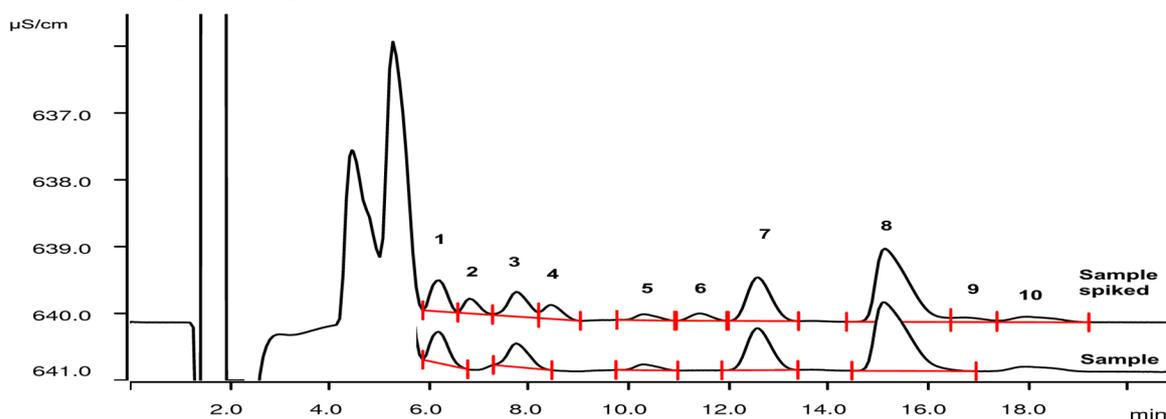
Cation chromatograms of a scrubber solution without spike (chromatogram partially shown, bottom) and with a spike of 0.5 mg/L amines (DMA [2], DEA [4], DPA [6], and DBA [9]). The recovery of the spikes was between 92–118%.
