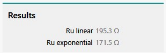
Figure 4 – The resistance values obtained from the linear and exponential fitting of the data
