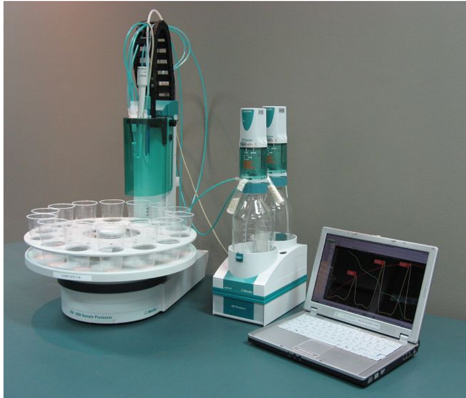
Automated Titrotherm system with sample processor
