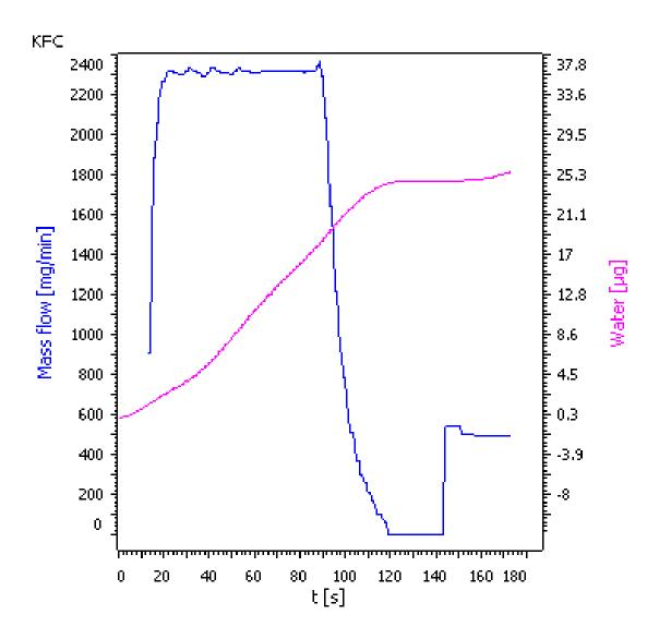
This Application Note describes the automated determination of the water content in liquid petroleum gas (LPG) and chloroethane using the 875 KF Gas Analyzer.
