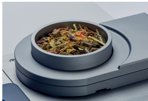
Analyzing rabbit food in diffuse reflection on the integrating sphere of the MPA II FT-NIR spectrometer.
