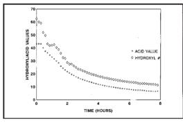
Figure 7. Summarized results from the application of NIR spectroscopy to the application of real time polyol process monitoring.
