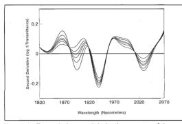
Figure 4. Expanded second derivative spectra of the polymeric combination O-H bands. Variation around 1900 nm corresponds to changes in the acid value, 1940 nm to changes in the moisture content, and 2030 nm to changes in the hydroxyl number.
