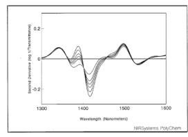
**Figure 3.** Expanded second derivative spectra of the polymeric first overtone O-H band. Variation around 1420 nm corresponds to changes in the hydroxyl number.
