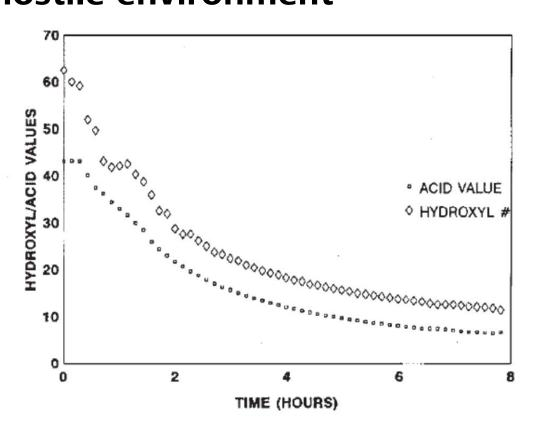
During polymerization, real-time determination of hydroxyl and acid numbers of polyols provide important information about the molecular weight and the reaction end point. This Application Note sheds light on the practical aspects of process monitoring in a polyol batch process using NIRS methodology. Real-time process monitoring with NIRS is the key to lower production costs and better product quality.
