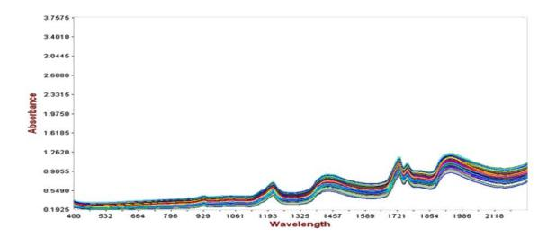
Near-infrared spectroscopy (NIRS) was used as an analysis method for quality control of soap noodles. Quantitative models for the determination of Total Fatty Matter, Iodine Number, and C8–C14 were developed, enabling fast and reliable quality control.
