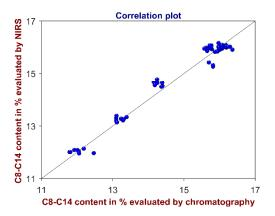
Fig. 5: Correlation plot of the C8–C14 content determined by chromatography and by NIRS.
