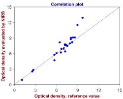
**Fig. 4:** Validation of the method for the determination of optical density. The correlation plot shows reference values versus optical density values evaluated by Vis-NIR spectroscopy. High coefficient of determination ( $R^2 = 0.9052$ ) and low standard error of prediction (SEP = 0.90) demonstrate that the method is suitable for its intended use.
