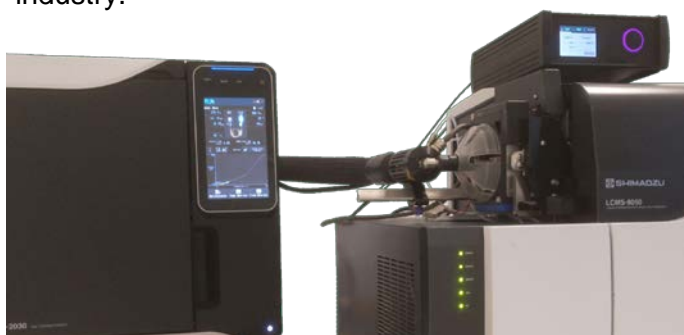
Figure 1: Coupling of GC-2030 and LCMS-8050 via SICRIT® ion source.
