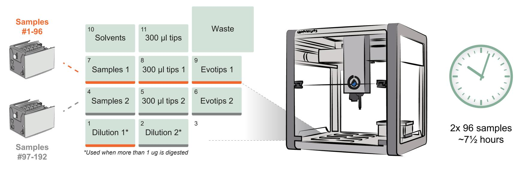
Layout of the Opentrons deck for automation of protein aggregation capture.
