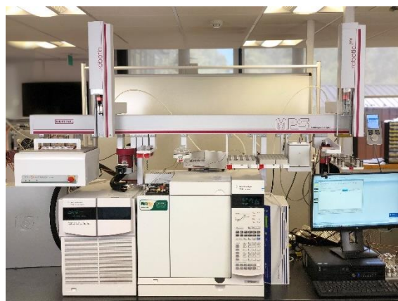
Figure 1: GERSTEL MultiPurposeSampler (MPS) used for nicotine extraction.
