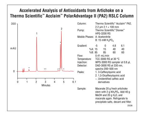
The Acclaim PolarAdvantage II column has better selectivity for these compounds than C18; the unknown and peak 2 coelute on C18. The RSLC column is three times faster and uses only 16% of the solvent, yet produces the same quality of chromatogram.
