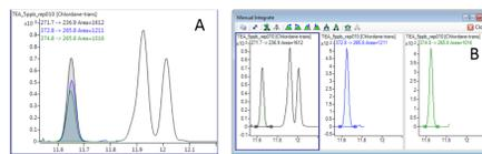
Figure 5. Trans-Chlordane at 5ppb in Tea: A) overlay of MRM transitions, and B) view of each transition separately.
