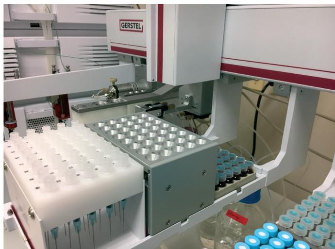
Figure 1. MPS robotic<sup>PRO</sup> sampler with the GERSTEL Fast Filtration Option.
