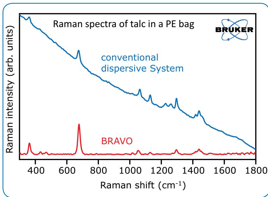
Raman spectra of talc in a PE bag measured with a conventional dispersive benchtop system and the BRAVO. BRAVO's SSE™ demonstrates efficient fluorescence mitigation and Duo LASER™ enables the detection of the weak Raman signals of talc with an exceptional signal to noise ratio.
