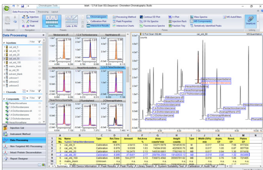
MS Quantitation channel (right) shows all XICs with SmartLink enabled for the MS Components pane (left).
