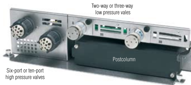
Figure 4b. The AM Automation Manager mounts inside the Detector Chromatography compartment (DC) and integrates up to two high-pressure valves, two solenoid valves, and a postcolumn heater. The entire AM mounts on a moveable slide for easy configuration for any application. All components are completely controlled through Chromeleon.
