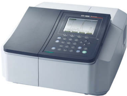
Shimadzu UV-1800 for measurement of beer color
