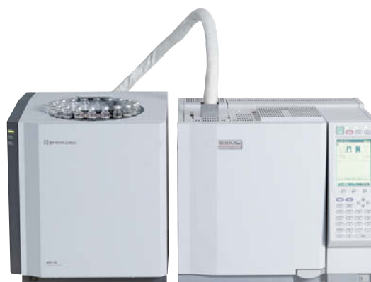
Shimadzu GC-2010 Plus or GC-2014 with HS-10 Headspace Autosampler for analysis of vicinal diketones
