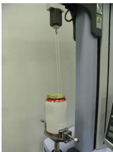
Tensile test on pull-tab on beer can containers with EZ-X
