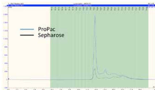
Figure 3. Gel filtration analysis of lysostaphin from ProPac and Sepharose IMAC columns. 50 mM \text{PO}_4 , 100 mM NaCl, pH 7.0 with a flow rate of 0.25 mL/min, 30 \mu\text{L} of the collected fractions injected, UV detection at 280 nm.
