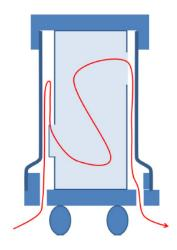
Figure 3. RapID Forced Air Cooling Vents
