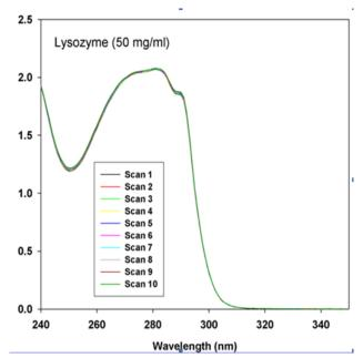
Although there is a very slight change due to evaporative loss over the course of this experiment, nearly 40 minutes elapsed between the first and last scans. This shows that the TrayCell has enough resistance to evaporative change to enable kinetic experiments to be performed.
