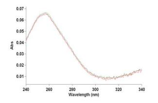
The results show the enhanced smoothness and precision of the Cary 300 despite the lower overall light throughput as a percent of normal beam. The reproducibility is within less than 1%. The precision of reading is slightly better than the Cary 50
