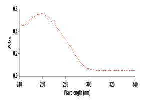
The scan is within the normal 'Concentrated DNA' PCR product range and the quantitative precision can be expected to be better than 99% for this concentration.
