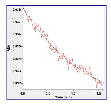
Results 9 Kinetics in Microvolumes A 4 ul Phosphite assay in a Traycell in Cary 4000
