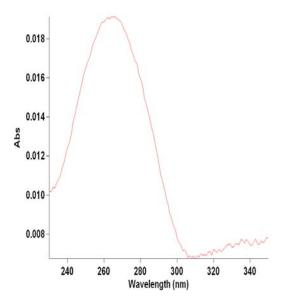
The optical performance of the Cary4000 far exceeds that of the Cary 50, however, in terms of DNA quantitation the error of 3-5% at 2ng/ul possible with the Cary 50 can be exceeded by the Cary 4000 but at these levels DNA quantitation is sufficiently precise for most analysis by Cary 50.
