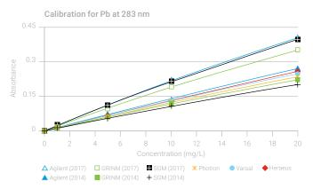
**Figure 5.** Comparison of calibration curves for lead (Pb) at 283.3 nm, based on tests conducted in 2014 and 2017. In each case, the Agilent lamp provided better sensitivity, especially at lower concentrations. The Agilent lead lamp tested in 2017 has an improved cathode composition, which explains the change in sensitivity from the lamp tested in 2014.
