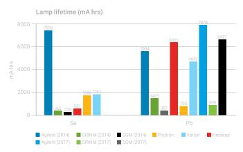
**Figure 16.** Lifetime of the selenium (Se) and lead (Pb) lamps. The Agilent lamp gave the longest life for both elements, well over 4 times longer than the nearest competitor for the Se lamp, and around 20% longer than the nearest competitor for the Pb lamp. The Agilent lead lamp tested in 2017 has an improved cathode composition, which improves both lifetime and performance compared with the lamp tested in 2014.
