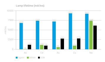
**Figure 17.** Lifetime for the arsenic (As), cadmium (Cd), gold (Au), copper (Cu) and sodium (Na) lamps. The Agilent lamp gave the longest life for each of these elements, well over 2.5 times longer than the nearest competitor for most elements, and >25% longer than the nearest competitor for the sodium lamp.
