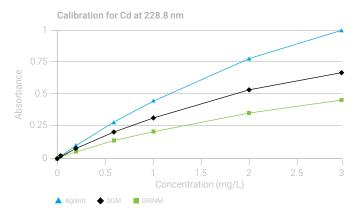
**Figure 10.** Comparison of calibration curves for cadmium (Cd) at 228.8 nm. The Agilent lamp provides the best sensitivity and linearity.
