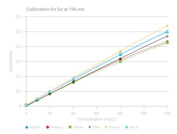
**Figure 6.** Comparison of calibration curves for selenium (Se) at 196.0 nm. The Agilent lamp ranks second in terms of sensitivity, comparable with the performance of the Varsal lamp. Only the Photron lamp provides better sensitivity, with similar detection limits.
