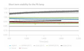
**Figure 13.** Short-term stability for lead (Pb) lamps, after a 10-minute warm up. While the Agilent and Heraeus lamps were suitably stable, the signals for both the Varsal and the GRINM lamps showed large spikes. The SGM lamps never appeared to stabilize.
