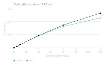
**Figure 7.** Comparison of calibration curves for arsenic (As) at 193.7 nm. The Agilent lamp shows slightly higher curvature when compared to SGM, however the Agilent lamp has better sensitivity at lower concentrations. GRINM lamps were also tested, but ceased operating before completion of the study.
