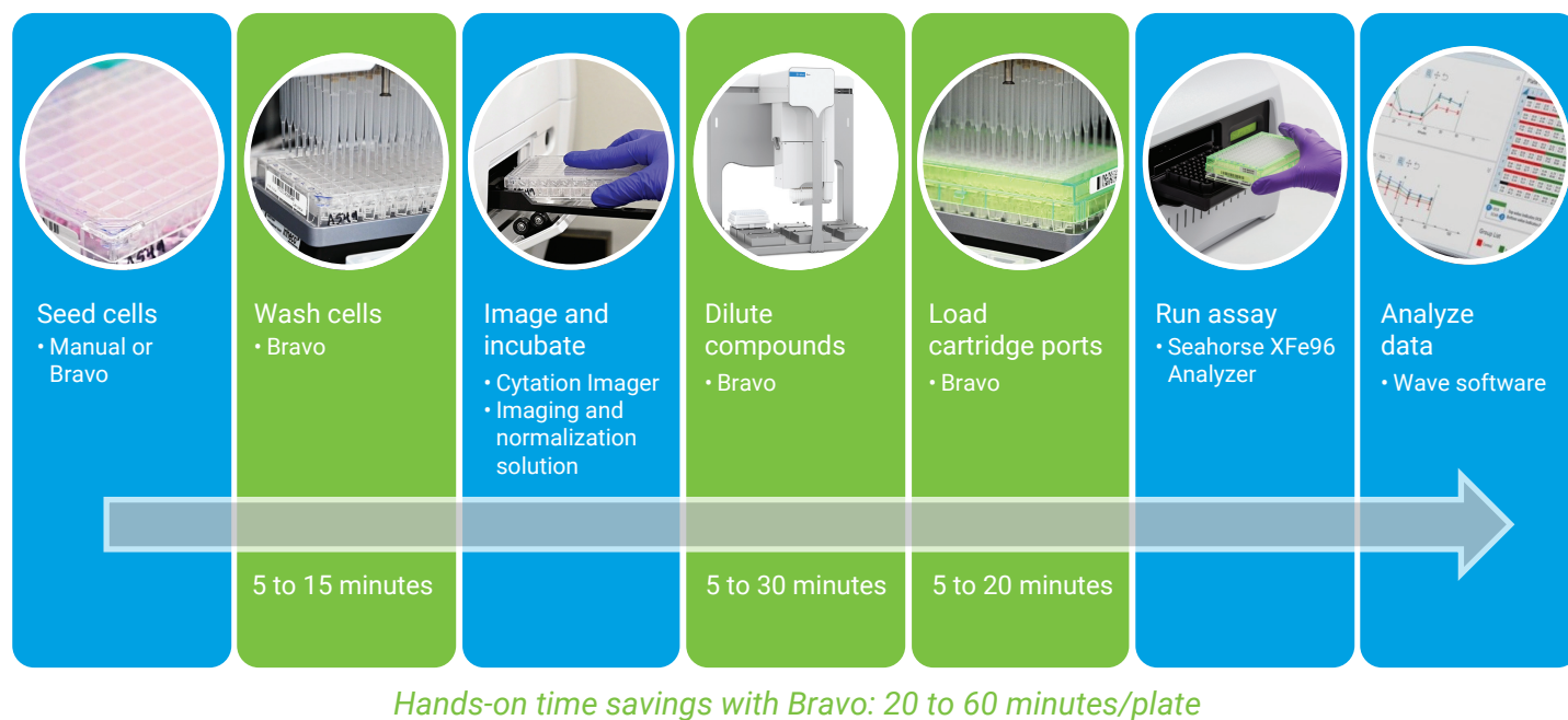
Figure 5. General Agilent Seahorse XF Assay workflow. Sample preparation steps automated with Bravo are shown in green: washing cells, preparation of injection solutions, and loading of Seahorse XFe96 sensor cartridges. Total hands-on time savings of 20 to 60 minutes per plate.
