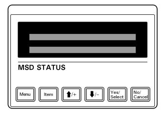
5973N and 5973 inert Mass Selective Detector Local Control Panel (LCP)
