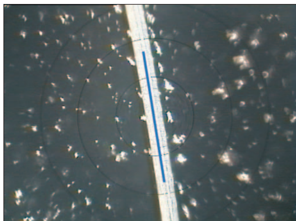
Figure 5: Optical image of the fiber in the analysis position. The blue line (1.7 mm long) indicates the position of the line scan.
