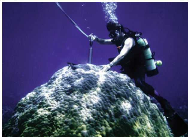
Figure 1. A diver drilling a Porites coral to obtain a core for geochemical analysis.
