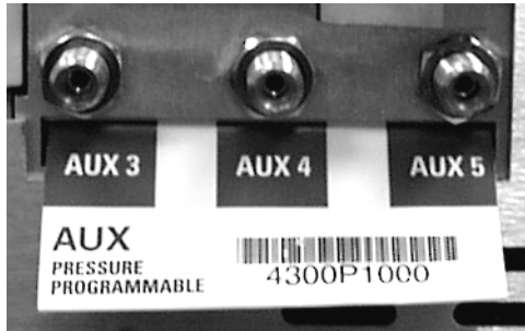
Figure 11 Gas line connections
