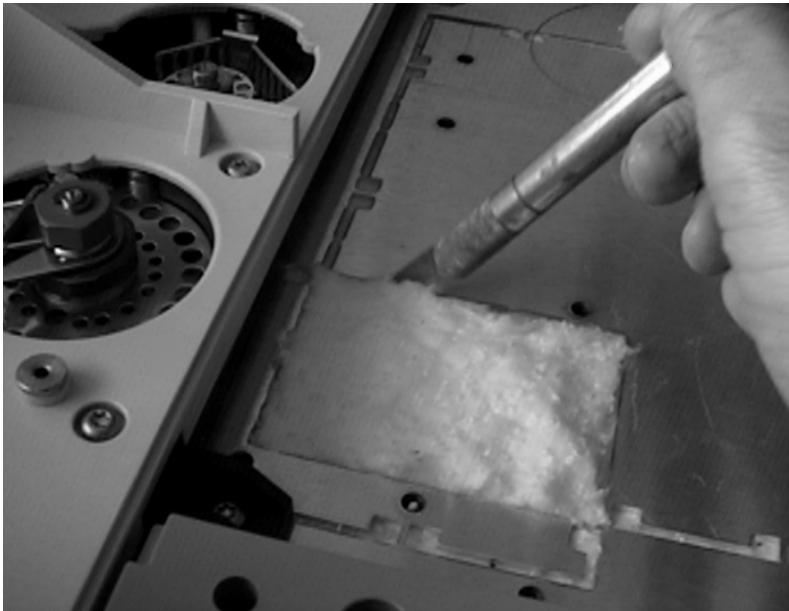
Figure 4 Cutting and removing the top layer of insulation
