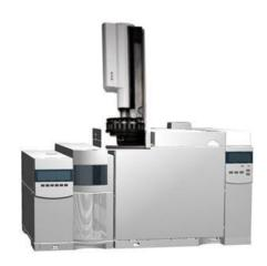
A simple system that includes a GC, an automatic liquid sampler, and a computer would require about 153 cm or 5 feet of bench space, add an addition 41cm for a LaserJet printer (195cm or about 6.5 feet); access to the MSD could require moving the instrument so an additional (30cm or 1 foot) should be available. A total of 244 cm or 8 feet of bench space should be available for a full GCMS system. Some repairs to the MSD or to the GC will require access to the back of the instrument.
