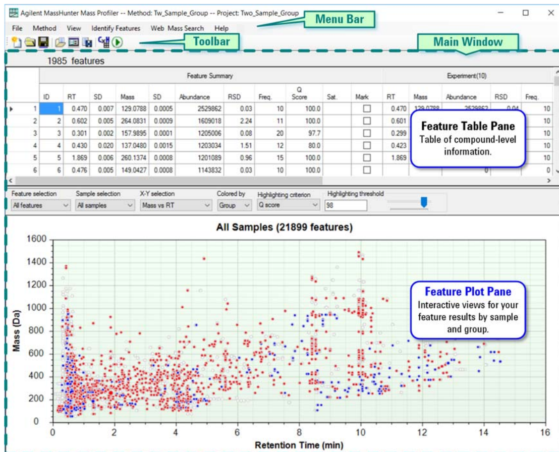
Figure 5 The main functional areas of Mass Profiler after a method is run on a project. If selected in the View menu, the Feature Plot can be replaced with a Features Details pane shown in Figure 6 on page 10.
