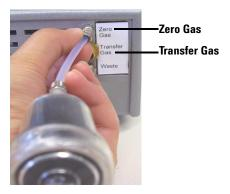
8 Remove the insulation and connect the Transfer Line.
