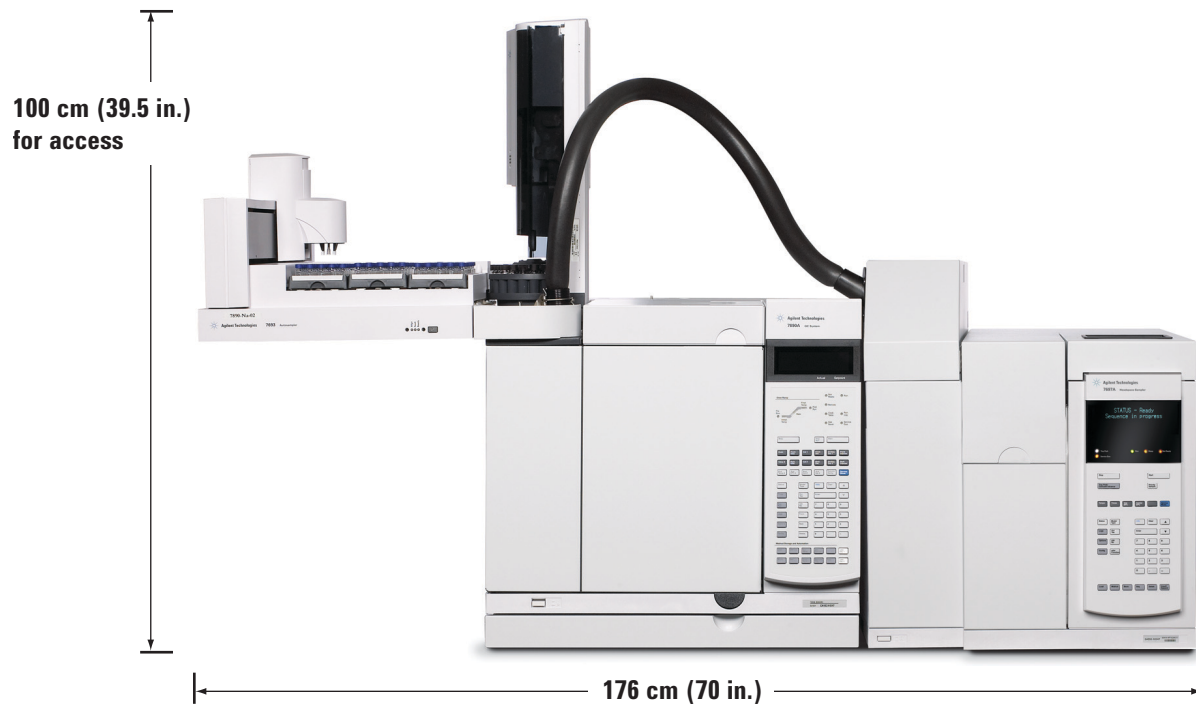
Figure 2 Example bench space needed for a 7890A GC–7697A HS system with 7693A ALS
