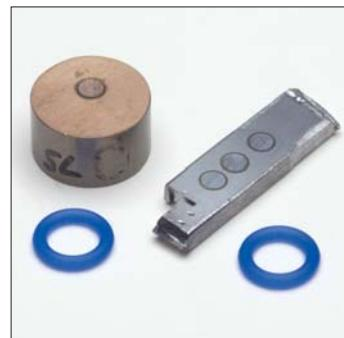
Preparation techniques that allow for analysis of extremely small sample types such as wires <1 mm in diameter and powder samples <320 mesh have been developed. The sample must be made larger by one of the techniques discussed below. The minimum final size of the sample must be 4.5 mm (4 mm anode) and 3 mm (2 mm anode).
