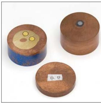
The entire mount can be made of the copper diallyl phthalate (PN 811-139); however, we find that using approximately 10 g to cover the sample is sufficient when backed by 5 g of the less expensive blue diallyl phthalate thermosetting powder (PN 811-135). The blue media does not soften with heat and resists the
