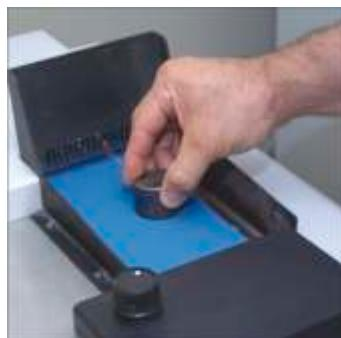
Avoid touching the analytical surface of the sample and the lamp. Wipe the anode with the foam wiper after the reaming cycle or just before mounting the next sample.
