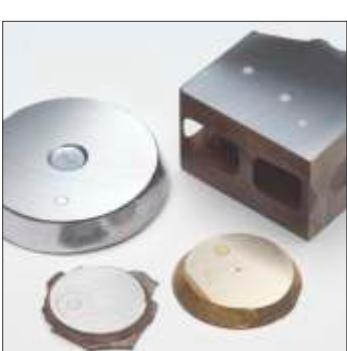
Disks should be analyzed close to the edge where rapid cooling has taken place. The top pour spout and bottom should be avoided. The correct amount of "skin" should be removed from the analytical face per ASTM guidelines; for example refer to ASTM Method E716-85EN for aluminum disks.
