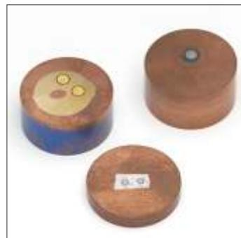
The entire mount can be made of the copper diallyl phthalate (PN 811-139); however, we find that using approximately 10 g to cover the sample is sufficient when backed by 5 g of the less expensive blue diallyl phthalate thermosetting powder (PN 811-135). The blue media does not soften with heat and resists the force of the reamer. The GDS900 cooling puck is always engaged which helps keep mounted specimens from over heating.
