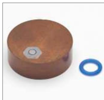
Preparation techniques that allow for analysis of extremely small sample types such as wires <1 mm in diameter and powder samples <320 mesh have been developed. The sample must be made larger by one of the techniques discussed below. The minimum final size of the sample must be 4.5 mm (4 mm anode) and 3 mm (2 mm anode).
